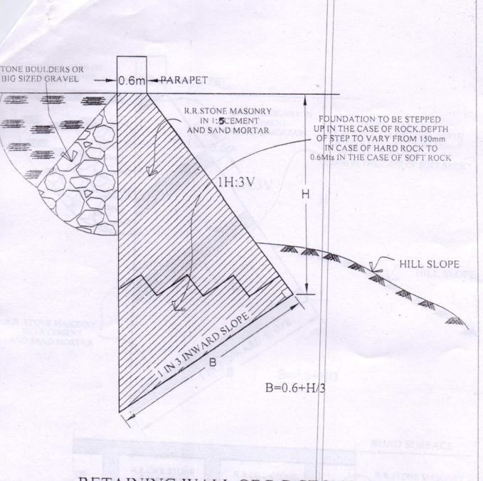
RETAINING WALL OF R.R STONE MASONRY IN 1:5 CEMENT AND SAND MORTAR
